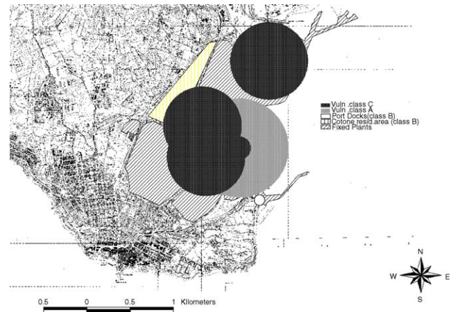
Fig. 10. Protection zones identified by the application of the Italian LUP criterion after hazard reduction actions.
